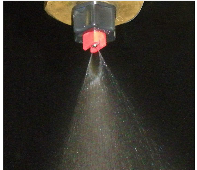
Fig. 6: Lubrication nozzle 652.185.16 at a spray pressure of 2 bar
