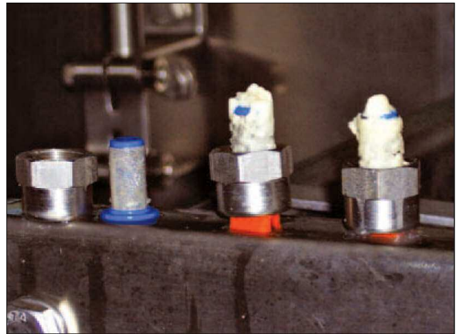
Fig. 9: Some synthetic belt lubricants have a high tendency for foam formation. This foam can accumulate on the strainer filter inserts of the nozzle and over time, lead to a blockage caused by slime [BRAUINDUSTRIE 2/2007]
