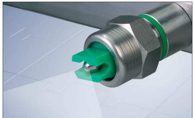
Fig. 2: Flat fan spray nozzles with a very small volumetric flow and a parabolic liquid distribution are used for conveyor belt lubrication [Ecolab]
