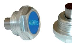
Consisting of a milled hexagonal head and crown in light aluminium alloy, the metal plug with magnet (which can also be used as a normal tank drain plug) can catch the metal particles present in the oil.
