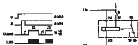
With pulse control and starting with pause (133)
