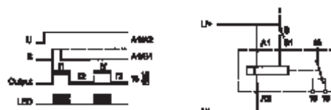
With pulse control and starting with pulse (134)
