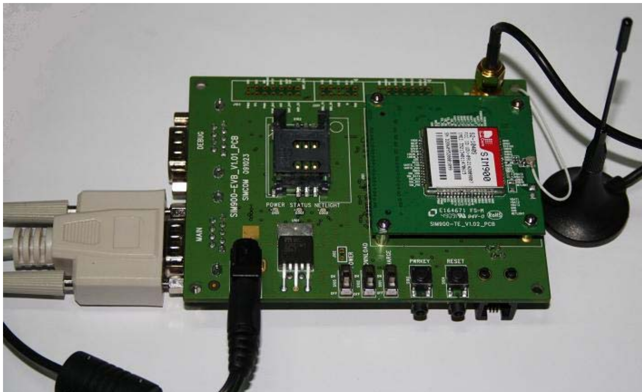
Figure 2: Top view of SIM900A EVB
