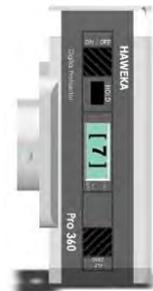
Step 8 Roll the unit so it faces away from you, the lettering should still read top to bottom. Align with same edge or line - wait 10 seconds. Press. HOLD-button until „[8]“ appears.
