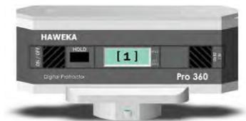
**Step 2** Rotate unit so it faces away from you, the lettering should still be right-side up.. Align with same edge or line, wait 10 seconds. Press HOLD-button until „[2]“ appears.
