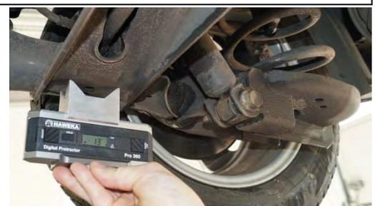
**5.3 Inclinometer with crown adapter and angle adapter
