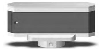
**Step 3** Roll unit so it faces you. The lettering should now be upside-down. Align with same edge or line - wait 10 seconds. Press HOLD-button until „[3]“ appears.
