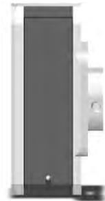
Step 7 Rotate unit end-for-end so it faces you, the lettering should now read top to bottom. Align with the same edge or line - wait 10 seconds. Press HOLD-button until „[7]“ appears.
