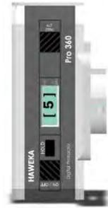
Step 6 Roll the unit so it faces away from you. The lettering should still read from bottom to top. Align with same edge or line - wait 10 seconds. Press HOLD-button until „[6]“ appears.
