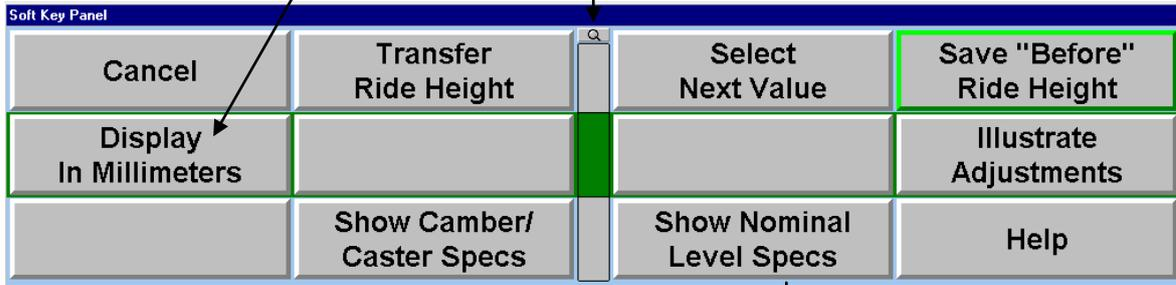
When choosing function *Show Nominal Level Specs*, the relevant nominal level specs for the selected vehicle can be shown as below (chart).
