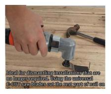
Ideal for dismantling installations that are no longer required. Using the universal E-CUT saw blades cut the rest part of nail on the wood.
