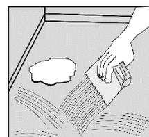
Lay the floor in the adhesive, following the technical data sheets and recommendations of adhesive producer.
