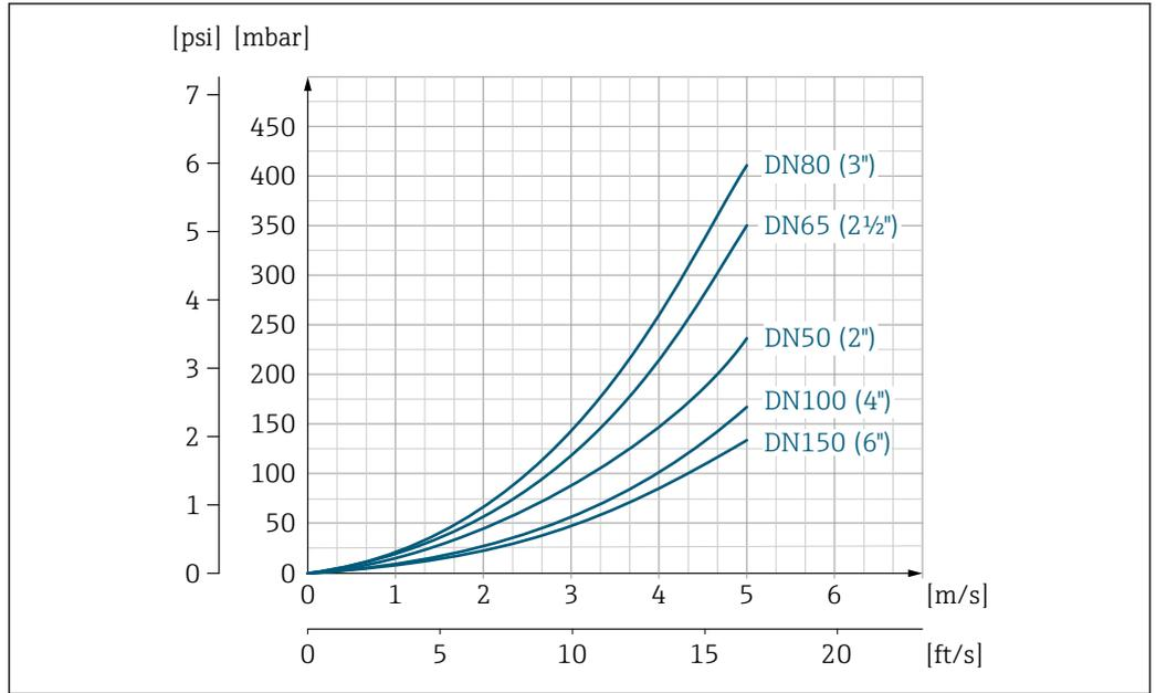
14 Pressure loss DN 50 to 150 (2 to 6")
