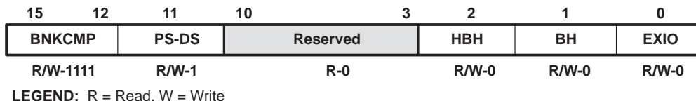
Figure 6. Bank-Switching Control Register (BSCR), MMR Address 0029h
