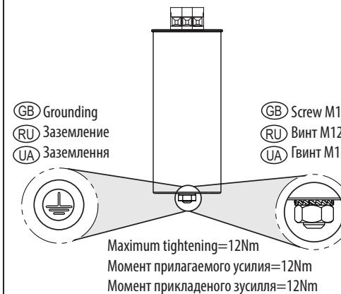
GB The capacitors can be mounted in horizontal or vertical position. If mounted horizontally ensure that the cooling is sufficient and additional mechanical fixing of the condenser is provided.
