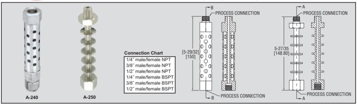
The Perforated and Spiral Cooling Towers protect pressure instruments during high temperature applications. Both the spiral and perforated styles are made with 316L stainless steel and are available with various process connections in NPT or BSPT style. Both Cooling Towers are ideal for use with pressure gages, switches, and transmitters where the process media temperature exceeds the rating of the instrument.
