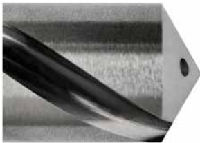
Drill flute insufficiently polished Rz = 0.45 µm
