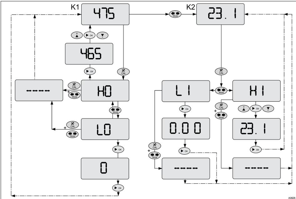
Fig. 25: ORP sensor calibration
