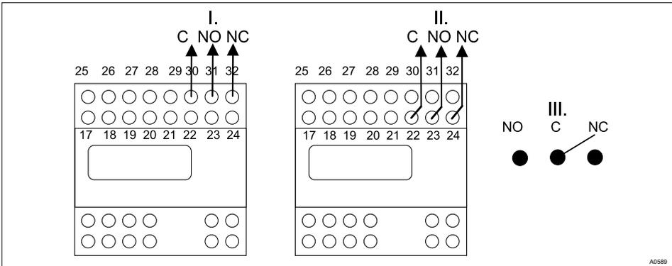
Fig. 7: Connection of the Relay Outputs
