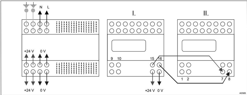
Fig. 4: Terminal diagram - DULCOPAC power supply
