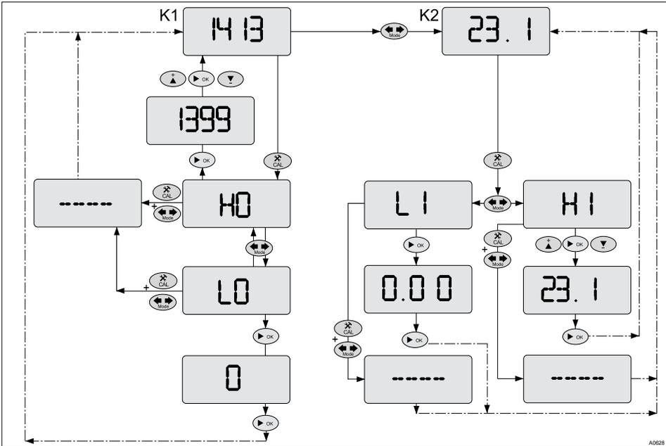
Fig. 27: Calibration of the measured variable conductivity
