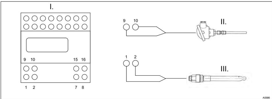
Fig. 5: pH sensor and temperature sensor (Pt 100)
