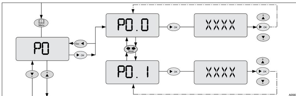
Fig. 12: P0 - Adjusting the setpoint
