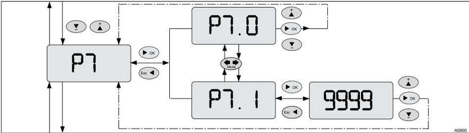
Fig. 19: P7 - Adjusting the digital inputs
