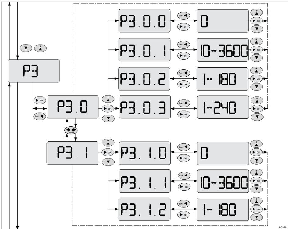
Fig. 15: P3 - Operating mode Adjusting the relay
