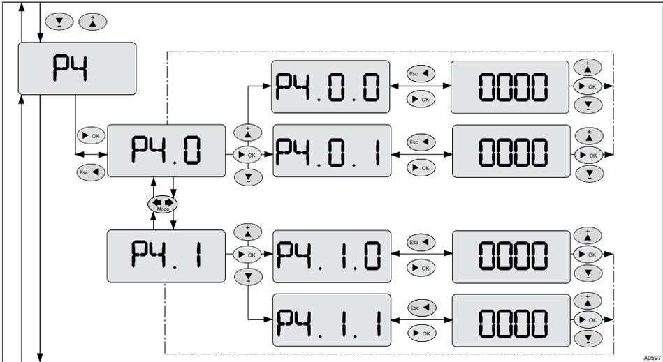
Fig. 16: P4 - Adjusting the alarm thresholds
