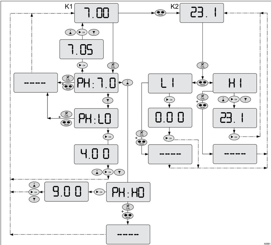
Fig. 24: Calibration of the measured variable pH and temperature
