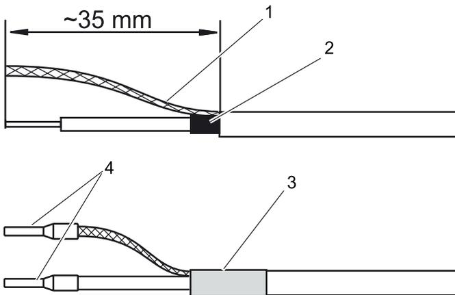
Fig. 8: Preparation of the coaxial cable
