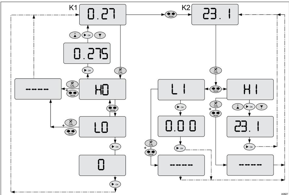
Fig. 26: Sensor slope calibration
