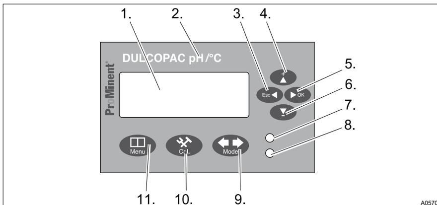
Fig. 9: Overview of device /Control elements
