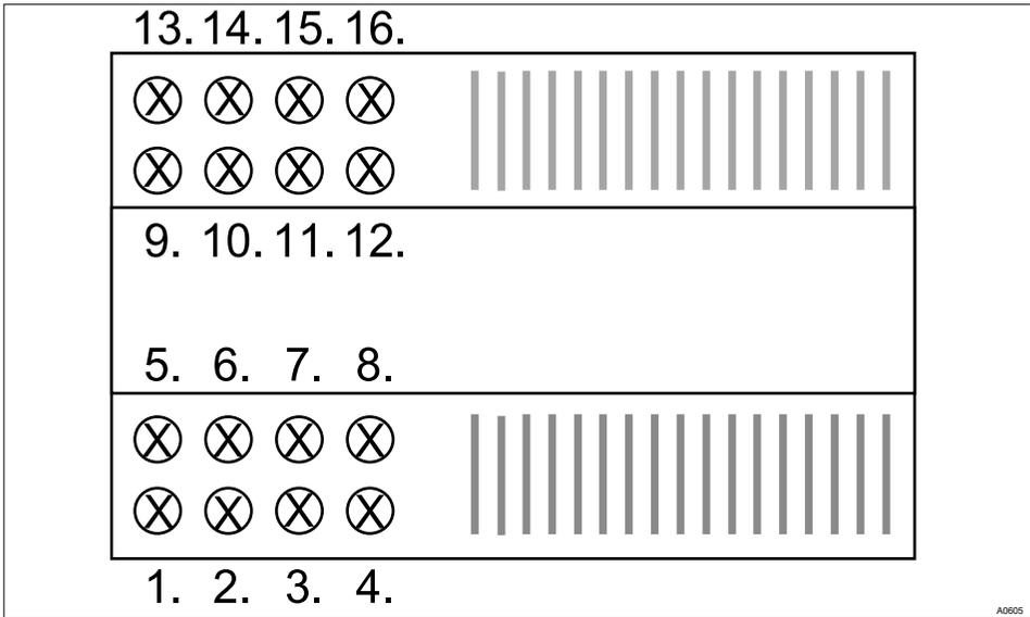
Fig. 2: Terminal allocation of the power supply module
