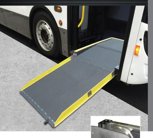
Unique cam-based design automatically adjusts platform to single continuous slope for easiest possible passenger access.
