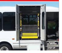
KlearVue<sup>™</sup> Model – Platform automatically and safely folds horizontally for unobstructed driver and passenger views. Accommodates longer lift platform inside a standard door opening, ideal for both side and rear-door applications.
