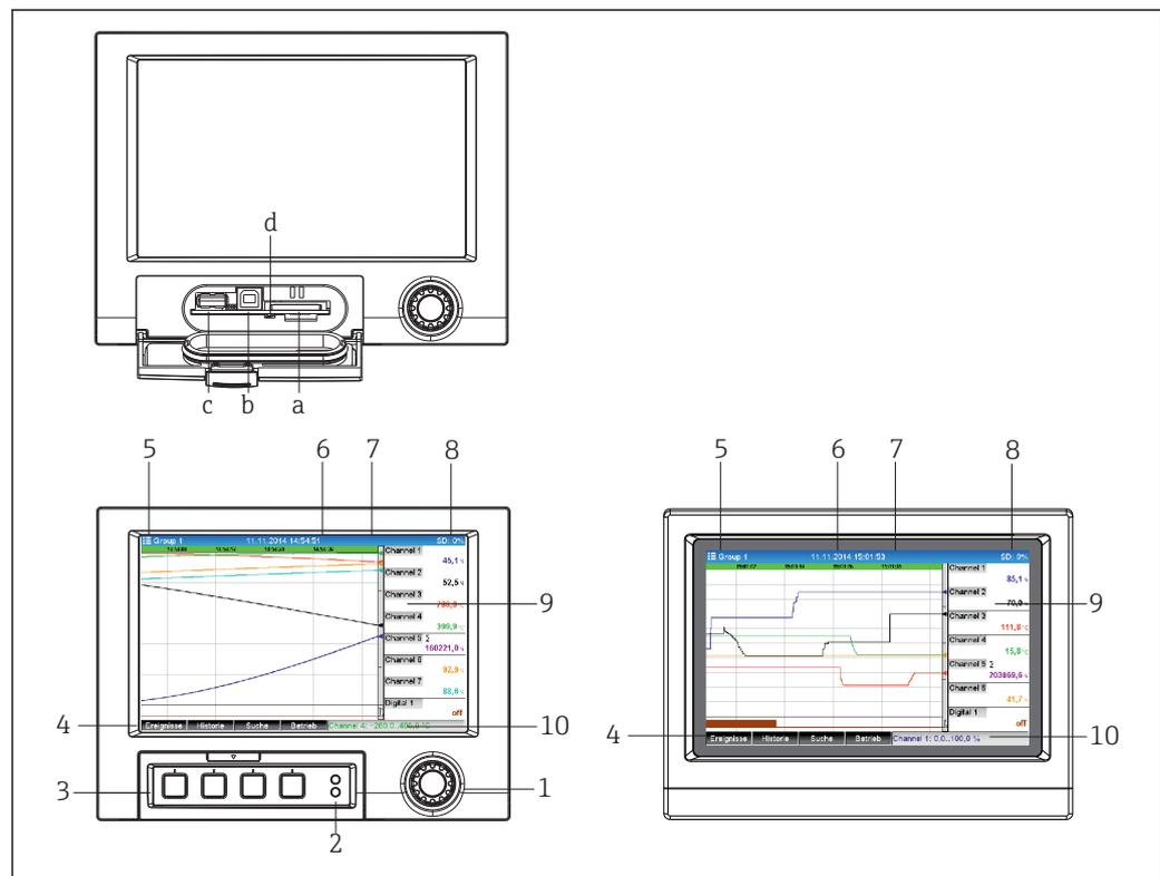
5 Device front (left: version with navigator and front interfaces; right: version with stainless steel front and touchscreen)
