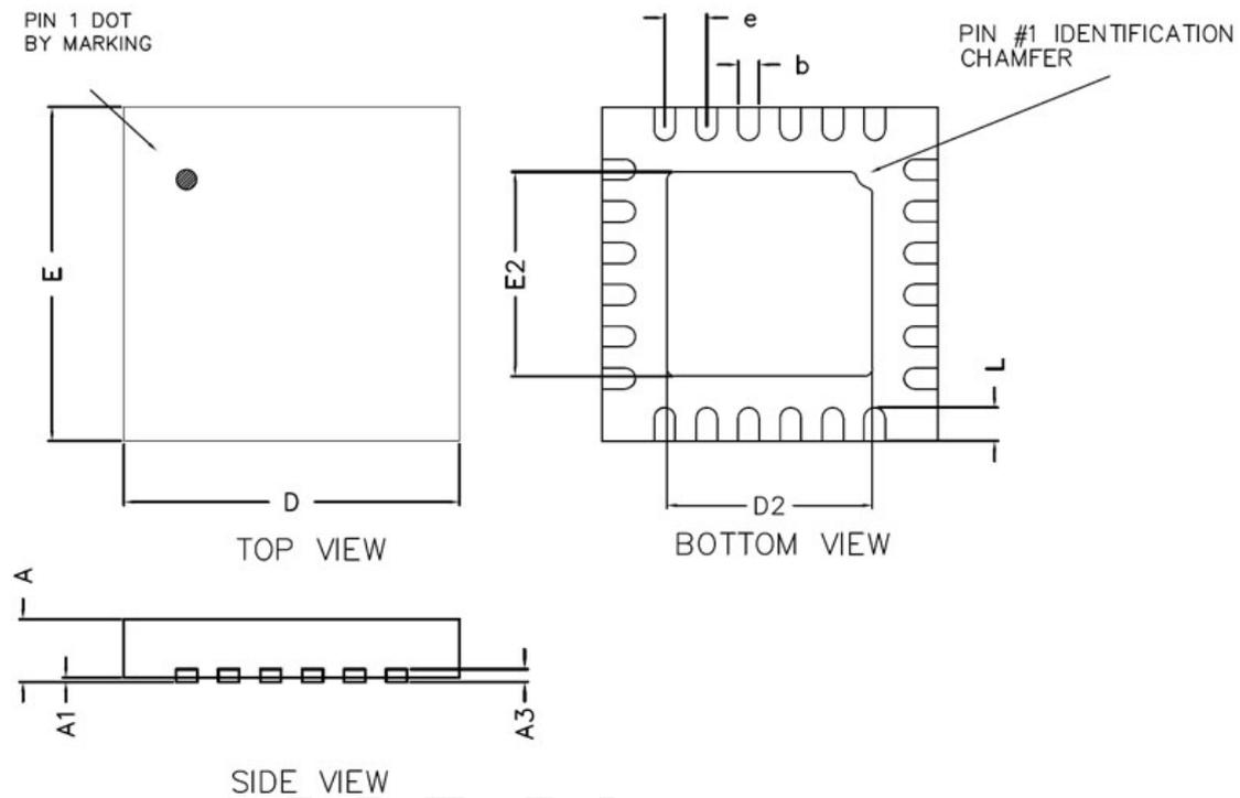
Figure 19 QFN 4x4 24 Pin Package diagram
