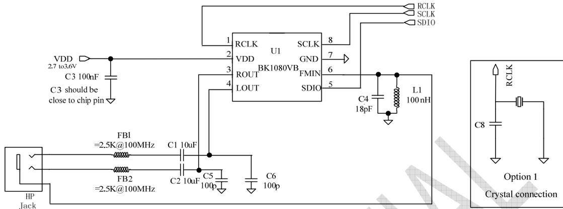
**Figure 18. BK1080VB with Single-ended Input Application**
