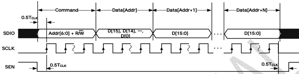
Figure 7 3-wire Interface Diagram
