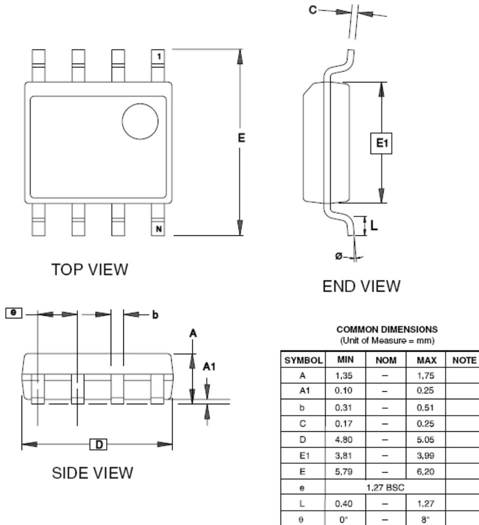
Figure 23 SOP 8 Pin Package diagram
