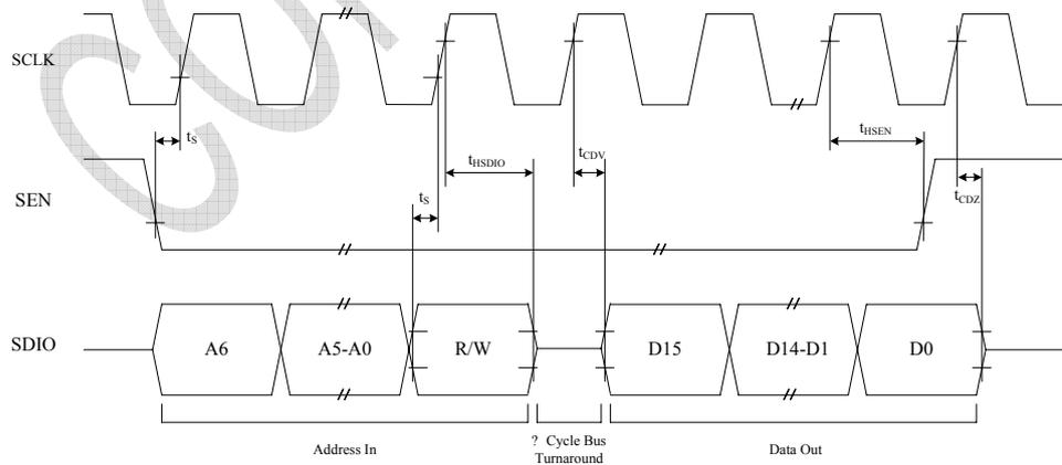
Figure 12 3-Wire Control Interface Read Timing Diagram
