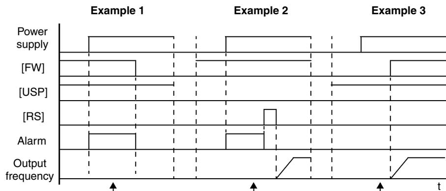
When USP is ON after powerup, the alarm (E13) will clear when the Run command (FW or RV) turns OFF.
