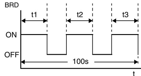
$$\boxed{\text{B90}} \text{ Duty cycle} = \frac{(t1 + t2 + t3 + \dots)}{100 \text{ seconds}} \times 100$$
