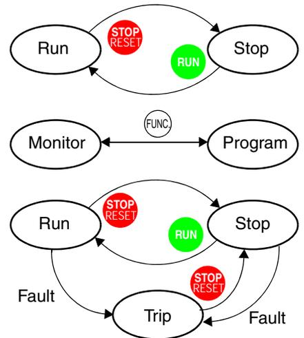
The occurrence of a fault during operation will cause the inverter to enter the Trip Mode as shown. An event such as an output overload will cause the inverter to exit the Run Mode and turn OFF its output to the motor. In the Trip Mode, any request to run the motor is ignored. You must clear the error by pressing the Stop/Reset switch. See [“Monitoring Trip Events, History, & Conditions” on page 6-5.](#)
