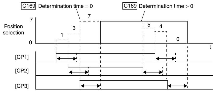
Note that excessively long determination time settings will reduce the overall performance of the position select inputs.
