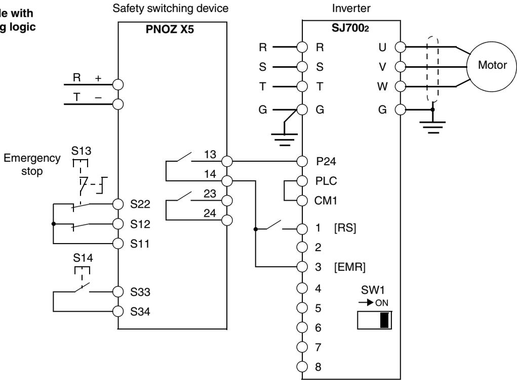
Example with sinking logic
