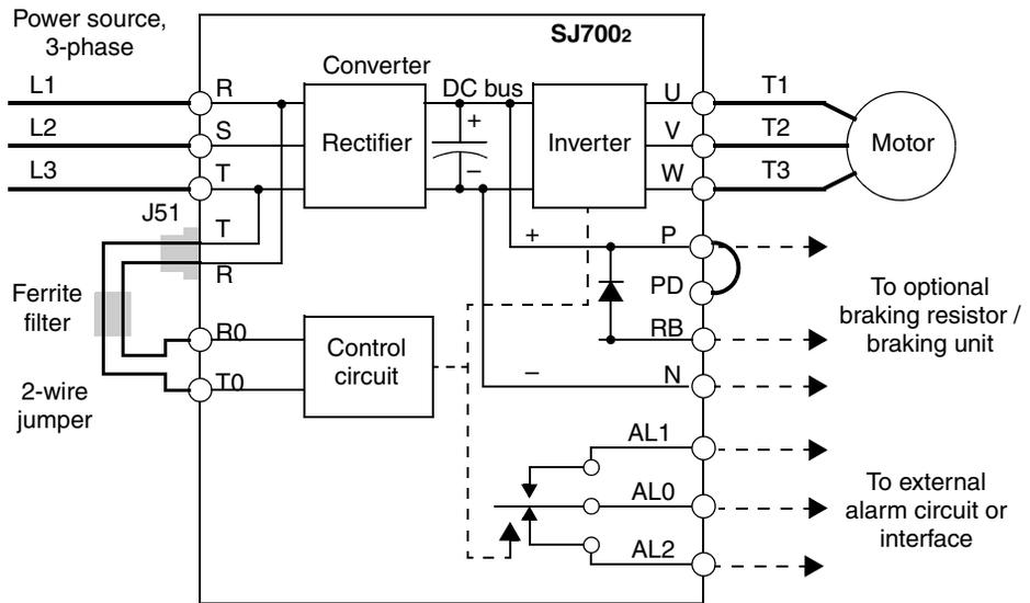
To provide power to the control circuit after input power loss, you must change the control circuit wiring as shown below (steps provided on following page).
