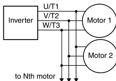
Some of the requirements when using multiple motors with one drive are:
