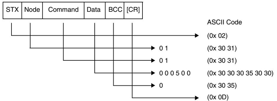
The block check code is computed by using the ASCII codes (shown above) and applying eXclusive OR (XOR) operations. Beginning with the first pair of bytes, the result of their XOR is then used in an XOR operation with the third byte, and so on. For this example, the BCC calculation is shown below.
