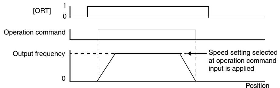
Teaching operation can be performed when power is input to the power supply terminals [R0] and [T0] of the inverter control circuit. The current position counter also operates when an external device moves the work piece. Therefore, the teaching operation can also be performed when the inverter does not operate (move) the machine.
