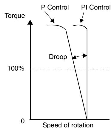
The proportional gain  $K_{pp}$  value determines the droop. Set the desired value using parameter H052. The relationship between the  $K_{pp}$  value and the droop is shown below:
