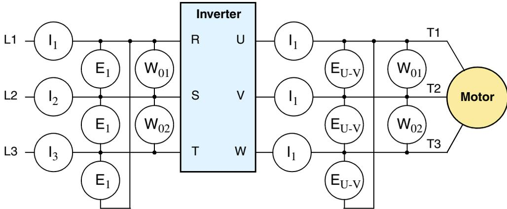
**Inverter Output Voltage Measurement Techniques**
