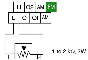
**Voltage Input** – The 0–10V voltage input circuit uses terminals [L] and [O]. Attach the signal cable’s shield wire to terminal [L] on the inverter only. DO NOT ground the shield at its other end. Maintain the voltage within specifications (do not apply negative voltage). Normally a full-span input level (10V) will give the maximum motor frequency. You can use parameter A014 to select a lower voltage for full output frequency (such as using a 5V input signal).
