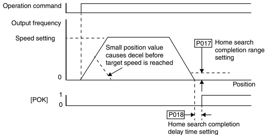
If zero return operation as described below is not performed, the motor position detected at powerup is assumed to be at the origin (position data = 0). When the operation command is turned ON with zero specified as the position setting, positioning is completed without running the motor.
