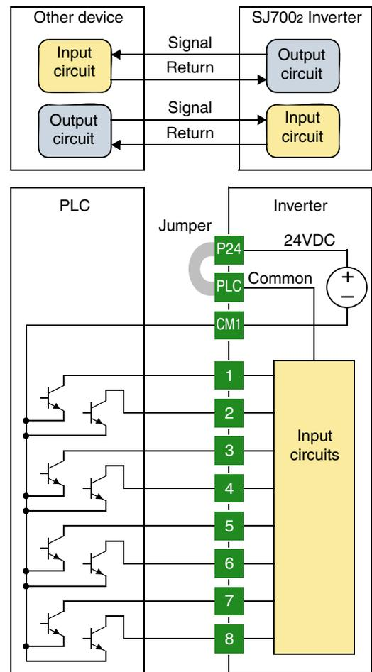
**Example Wiring Diagram**
