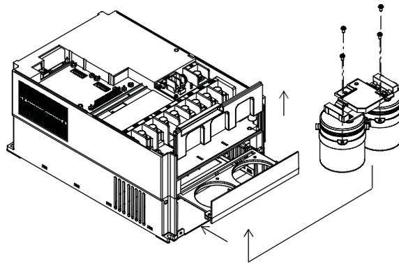
To install the new capacitor unit:
