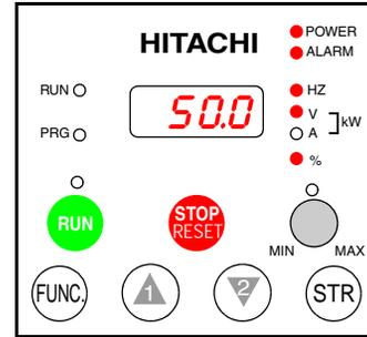
For the powerup test, monitor the motor speed indirectly by viewing the inverter's output frequency. The *output frequency* must not be confused with *base frequency* (50/60 Hz) of the motor, or the *carrier frequency* (switching frequency of the inverter, in the kHz range). The monitoring functions are in the "D" list, located near the top left of the diagram in the ["Keypad Navigational Map" on page 2-31](#).
