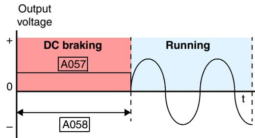
If an inverter is started into such a backward-rotating load, over-current trips can occur. Use DC braking as an “anti-windmilling” technique to stop the motor and load, and allow a normal acceleration from a stop. See also the [“Acceleration Pause Function” on page 3-21](#).
