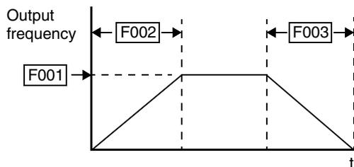
Acceleration 1 and Deceleration 1 are the standard default accel and decel values for the main profile. Accel and decel values for an alternative profile are specified by using parameters Ax92 through Ax93. The motor direction selection (F004) determines the direction of rotation as commanded only from the keypad. This setting applies to any motor profile (1st, 2nd, or 3rd) in use at a particular time.
