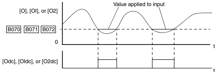
The inverter can also detect when an analog input value is within a range (or *window*) of values. See [“Window Comparator Signals” on page 4-62](#).
