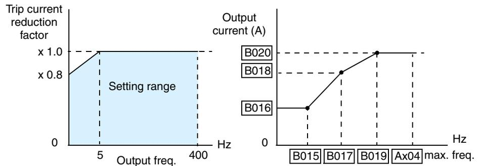
Suppose the electronic thermal setting (B012) is set to 44 Amperes. The graph below shows the effect of the free setting torque characteristic curve. For example, at (B017) Hz, the output current level to cause overheating in a fixed time period is reduced to (B018) A. Points (x), (y), and (z) show the adjusted trip current levels in those conditions for given trip times.
