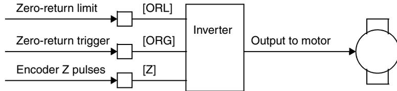
The three available zero-return modes differ in the overall search speed, final approach direction to the origin, and the limit switch input transition (or encoder pulse, if used) causing the final stop. Choose the zero-return mode that best fits your application.
