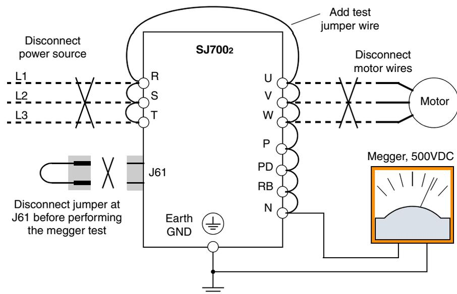
7. After completing the test, disconnect the megger from the inverter.
