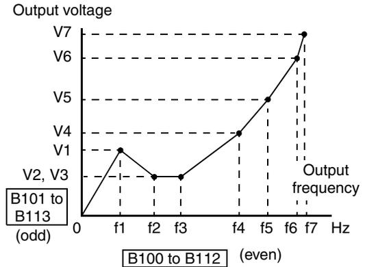
**NOTE:** The using of V/f free-setting operation specifies parameters that override (make invalid) certain other parameters. The parameters that become invalid are torque boost (A041/A241), base frequency (A003/A203/A303), and maximum frequency (A004/A204/A304). In this case, we recommend leaving their settings at the factory default values.
