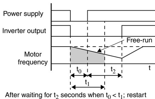
**Example 2: Power failure longer than limits; trip**
