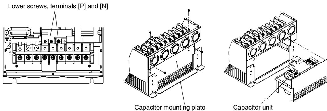
To install the new capacitor unit:
