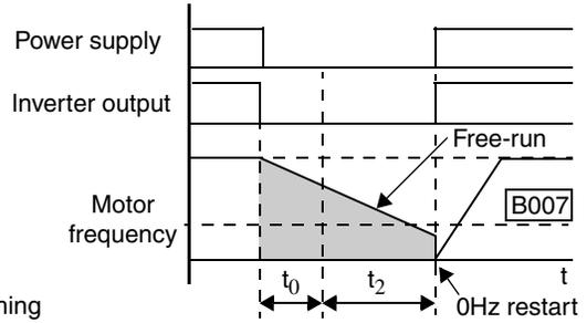
Motor frequency < B007 value at  $t_2$
