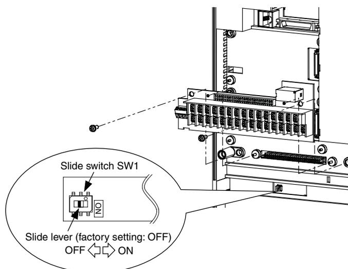
When the emergency stop function is enabled, intelligent input terminals [1] and [3] are used exclusively for this function, and no other functions can be assigned to these terminals. Even if other functions have been assigned to these terminals, these are automatically disabled and these terminals are used exclusively for the emergency stop function.
