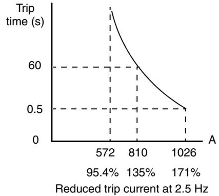
**Free Thermal Characteristic** - It is possible to set the electronic thermal characteristic using a free-form curve defined by three data points, according to the table below.
