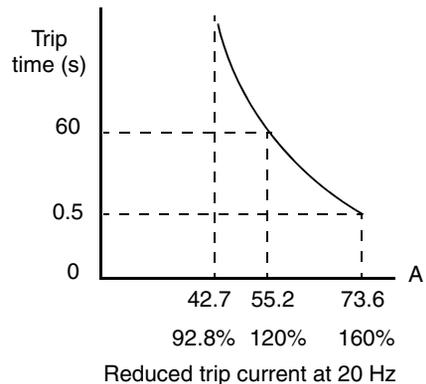
**Constant Torque Characteristic** – Selecting the constant torque characteristic for the example motor gives the curves below. At 2.5 Hz, the output current is reduced by a factor of 0.9 for given trip times.
