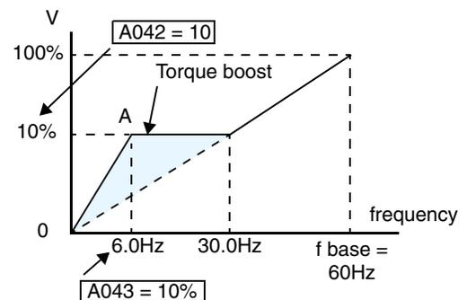
Be aware that running the motor at a low speed for a long time can cause motor overheating. This is particularly true when manual torque boost is ON or if the motor relies on a built-in fan for cooling.
