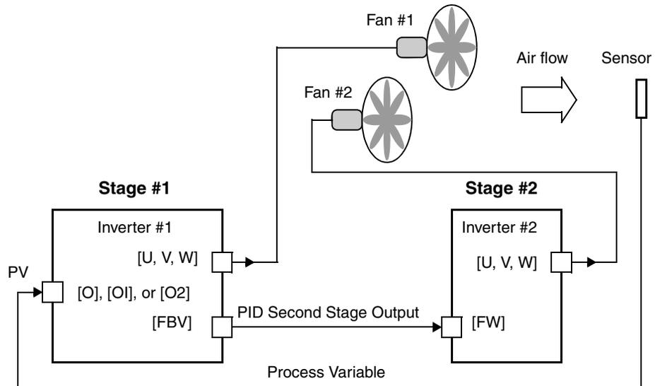
**NOTE:** The [FBV] is designed for implementing two-stage control. The PV high limit and PV low limit parameters, C052 and C053, do not function as process alarm thresholds. Terminal [FBV] does not provide a PID alarm function.
