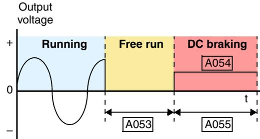
**When starting** – You can also apply DC braking upon the application of a Run command, specifying both the DC braking force level (A057) and the duration (A058). This will serve to stop the rotation of the motor and the load, when the load is capable of driving the motor. This effect, sometimes called “windmilling,” is common in fan applications. Often, air moving in duct work will drive the fan in a backward direction.
