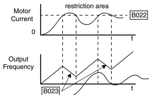
When the inverter detects an overload, it must decelerate the motor to reduce the current until it is less than the threshold. You can choose the rate of deceleration that the inverter uses to lower the output current.
