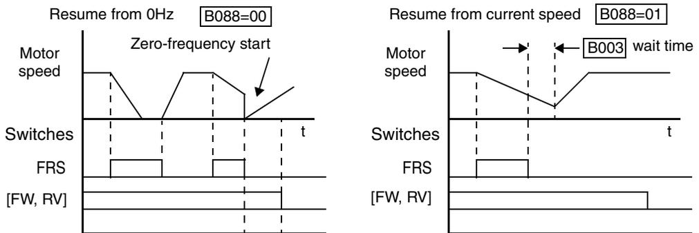
In the diagram above, [FRS] signal is active high. If you want the [FRS] terminal to be active low (normally closed logic), change the setting (C011 to C018) that corresponds to the input [1] to [8] that is assigned the [FRS] function (C001 to C008).
