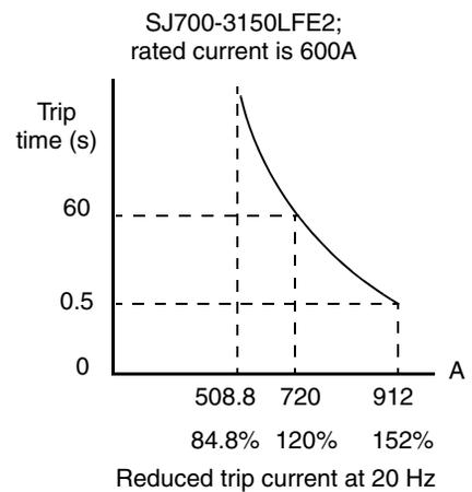
**Constant Torque Characteristic** – Selecting the constant torque characteristic for the example motor gives the curves below. At 2.5 Hz, the output current is reduced by a factor of 0.9 for given trip times.
