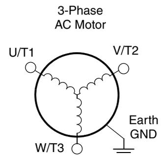
Notice the three connections to the motor do not include one marked “Neutral” or “Return.” The motor represents a balanced “Y” impedance to the inverter, so there is no need for a separate return. In other words, each of the three “Hot” connections serves also as a return for the other connections, because of their phase relationship.
