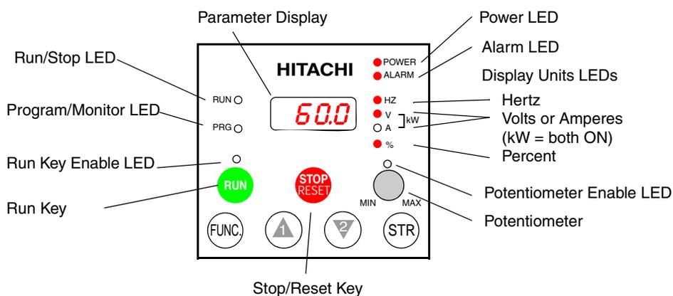
The display is used in programming the inverter's parameters, as well as monitoring specific parameter values during operation. Many functions are applicable only during the initial installation, while others are more useful for maintenance or monitoring.
