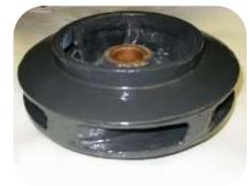
Impeller from a sea water pump was badly eroded. The pump was obsolete and no spare parts were available. The surface of the impeller was rebuilt using 301 Epoxy Resin with glass fillers and then machined to a smooth finish. Once cured 2 coats of 202 Ceramic Repair Fluid was applied to all of the impeller to complete the repair
