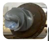
Impeller for a large water pump has become badly eroded and required resurfacing. The impeller was abrasive blast cleaned and 2 x coats of 202 Ceramic Repair Fluid applied to the surface
