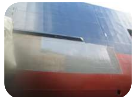
Corroded bow on large container vessel abrasive blast cleaned and filled using 101 Metal Repair Paste
