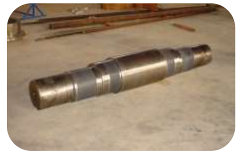
Shaft on stone crusher damaged and worn. Surfaces were rebuilt using 101 Metal Repair Paste and machined on a lathe to bring the shaft surface back to the original factory finish
