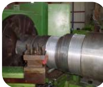
Shaft on stone crusher damaged and worn. Surfaces were rebuilt using 101 Metal Repair Paste and machined on a lathe to bring the shaft surface back to the original factory finish
