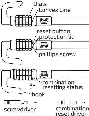
Adjustable pedal to steering wheel anti-theft device with combination lock "WheelBlock PRO"
