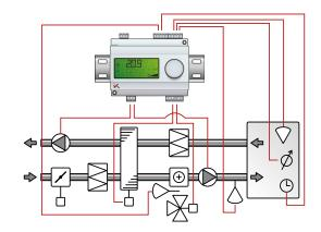
This control mode requires two sensors, "Supply air sensor" on AI1 and either "Room sensor" or "Extract sensor" on AI2.
