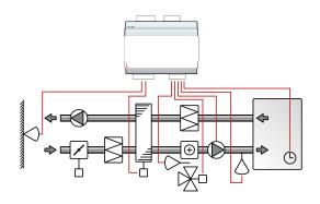
This control mode requires a sensor, "Supply air sensor", on AI1.
