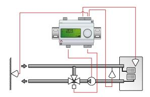
This control mode requires two sensors, "Supply temperature" on AI1 and "Outdoor sensor" on AI2.
