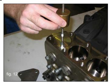
A) Unfasten the 7 M12x35 valve cover screws, and remove the cover, fig. 12.
