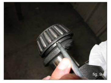
The new roller bearing can be mounted at room temperature with a press or fly press; it is necessary to lay them on the lateral side of the relevant ring nuts with apposite rings. The driving operation can be facilitated by heating the relevant parts at a temperature ranging between 120° - 150° C (250° - 300° F), making sure that the ring nuts are correctly fitted into their seats.
