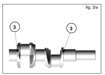
C) Disassemble the crankshaft oil seals and the piston guides using standard tools.
