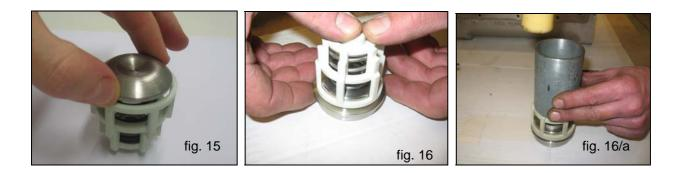
Insert the suction and delivery valve units checking that they are thoroughly inserted in the head seat. Therefore apply the valve covers and proceed with calibrating the related M12x35 screws with a torque wrench as indicated in Chapter 3.
