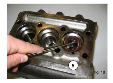
Pay careful attention to the order of sealing pack disassembly as shown in fig. 19, composed of: 1. Head ring
