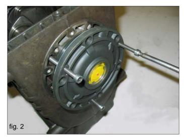
B) Push the piston guides and connecting rods forward in order to facilitate the lateral extraction of the pump shaft.
