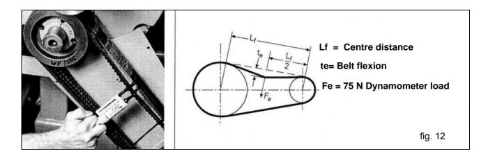
$N.W_1$ . If not differently indicated by the belt Manufacturer, the inspection of the correct tension value, and the related tension adjustment if needed, is to be carried out after at least 30 minutes of operation in order to obtain belt settling. The best efficiency and maximum duration is obtained with the correct tension value.
