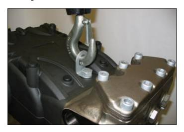
In case of disassembly, to avoid letting filth inside the front part of the crankcase, close the threaded hole with the supplied cap.
