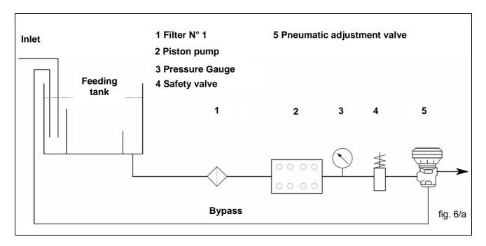
The filter must be installed as close as possible to the pump, should allow easy inspection and have the following characteristics:
