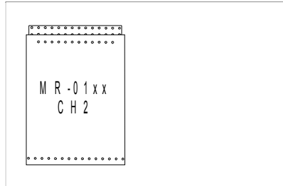
Fig.7.1 Placement of a plug-in submodule with serial interface onto the middle board of the basic module
