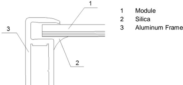
The depth is no less than 3mm when installing the module into the frame.
