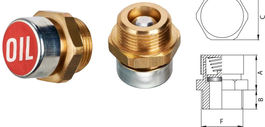
The breather plug with valve proposed here works on the following principle: venting is obtained by the pressure inside the reducer acting on the closing gasket, which raises the spring preset to a pressure of 0.25 - 0.30 bar allowing the vapours to escape and then closes.
