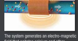
field that agitates calcium and other minerals in the water, causing them to create suspended crystals.
