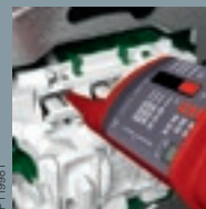
Measuring holes in the front
