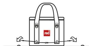
Connect all four clips to the Cargo Point D-Rings located on the front of the board
