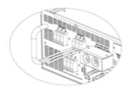
The inverter is equipped with several communication ports and it is also equipped with a slot for alternative communication interfaces in order to communicate with a PC with corresponding software. This intelligent slot is suitable to install with SNMP card and Modbus card. Follow below procedure to connect communication wiring and install the software.
