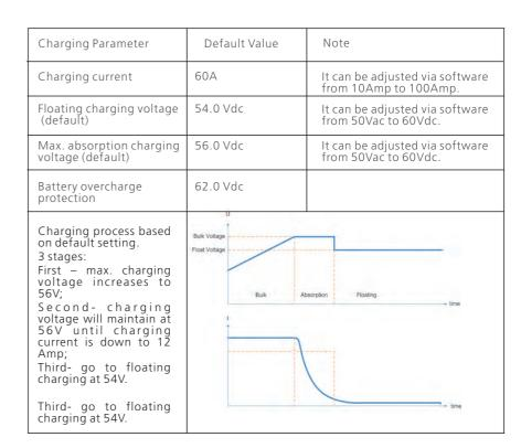
This inverter can connect to battery types of sealed lead acid battery, vented battery, gel battery and lithium battery. The detail installation and maintenance explanations of the external battery pack are provided in the manufacturer's external battery pack of manual.
