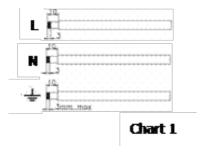
Step 4: Connect wires according to polarities indicated on terminal block. Be sure to connect PE protective conductor (((-)) first.
