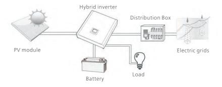
Figure 1 Basic hybrid PV System Overview
