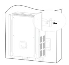
4.Check if the inverter is firmly secured.
