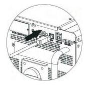
For SNMP or MODBUS card, you should use RJ45 cables as follows:
