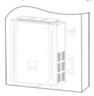
3. Fix the inverter in position by screwing the supplied two screws (M4\*12) located on the top two sides of the inverter.
