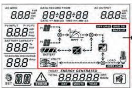
Real-time operation status Section 12-5 describes all operation conditions when the inverter is set up at "Grid-tie with backup (I)"
