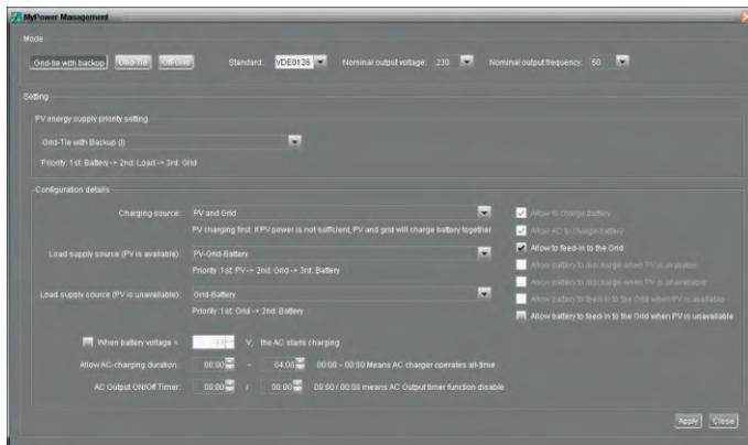
PV energy supply priority setting: 1st Battery, 2nd Load and 3rd Grid.
