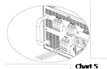
Step 3: Make sure the wires are securely connected. The reference tightening torque is 0.82 N.m.
