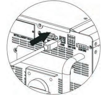
For Dry contact port, please remove insulation sleeve 8 mm for three conductors and insert three cables into ports
