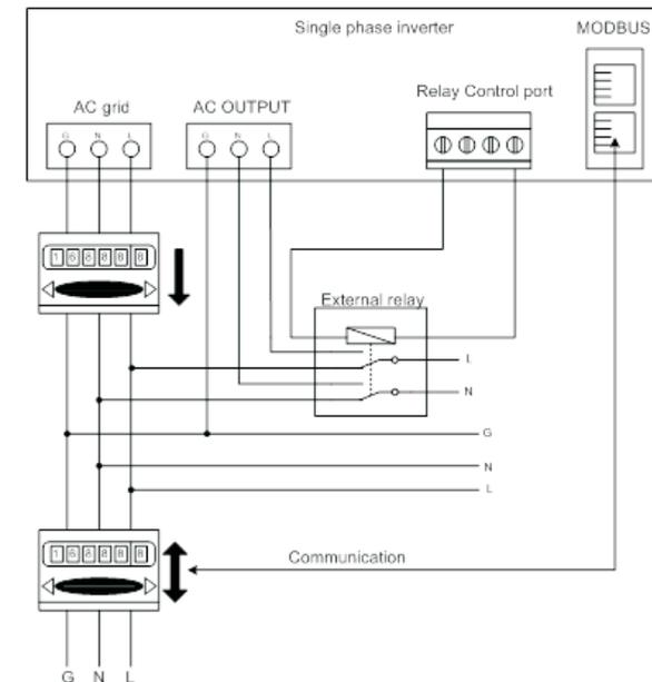
With Modbus card II and energy meter, hybrid inverter can be easily integrated into the existing household system. For details please refer to Modbus card II manual.
