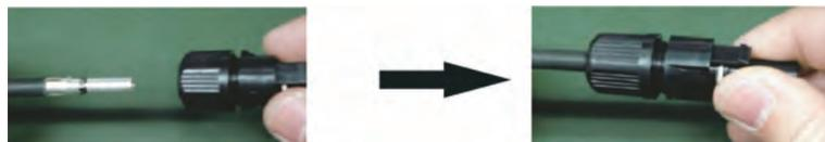
Insert striped cable into male terminal and crimp male terminal as shown below charts.
