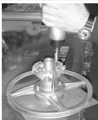
Fix the nuts (ref. 23/b) over the bolts. Tighten the nuts by using pneumatic screw-driver (ref.36/b).
