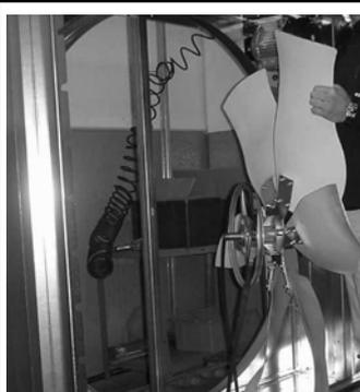
Tighten bolts , washers (ref. 25/b) and nuts (ref. 25/c) in order to fix the centrifugal system to the propeller by using pneumatic screw-driver (ref.36/ d). Place the complete assembly you have obtained on the fan, inserting the axle trough the central support hole.
