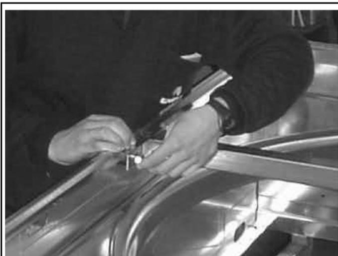
Place the oval plate over support frame and then start to screw the nuts.
