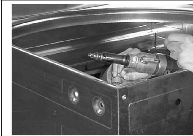
Place the qty. 2 short threaded bushes (ref. 19/a) on the top panel by using inserting machine (ref. 35).
