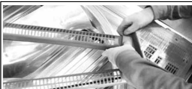
Join the plastic safety protection for the motor pulley.
