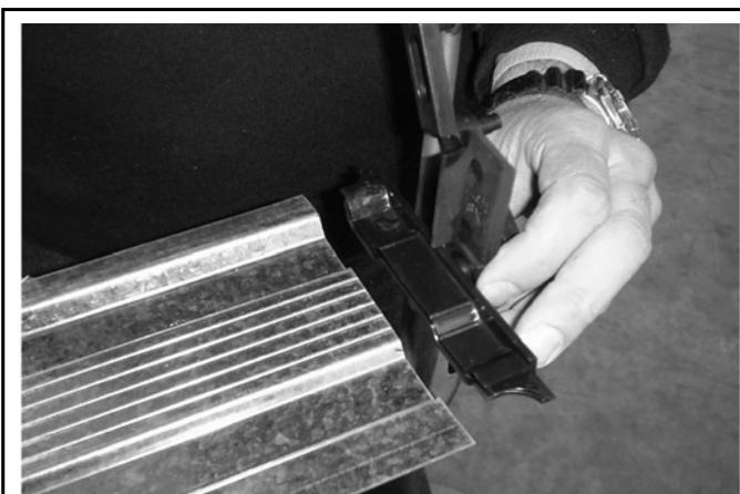
Insert plastic bearing with spring (ref. 14/c , 14/d) on central shutter blade (ref.6/b)."SX" is for left side, "DX" is for right side. Fix the plastic fork (ref.27/a) with qty. 2 bolts (ref.27/b) and qty. 2 nuts (ref. 27/c) on the central shutter blade.
