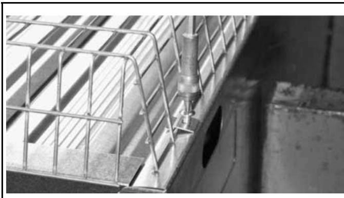
Fix it to the bottom and top panels by means of qty. 6 metal clips (ref. 17/b) and qty. 6 screw (ref. 17/b). The metal clips must be fixed in the position as in the picture.
