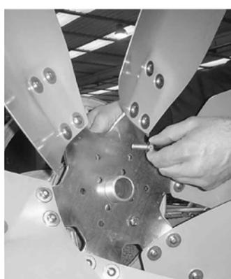
Place the propeller (ref. 5) on the central pulley assembly. Fix the bolts (ref.24/a), the washers (ref. 24/b) and nuts (ref. 24/c) in order to fix the propeller.
