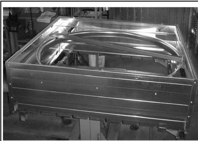
The propeller central support (ref. 12) shall be fixed to housing by means of qty. 4 bolts (ref. 21/a), qty. 4 washes (ref.21/b), qty. 4 nuts (ref.21/c) and qty. 2 oval plates (ref. 21/d).
