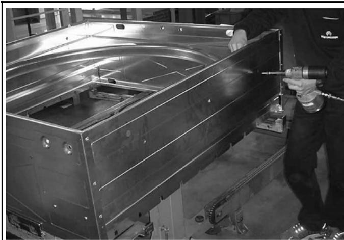
Place long threaded bushes (ref. 19/b) in correspondence of proper holes around the housing. Qty. 2 long threaded bushes for each panel.
