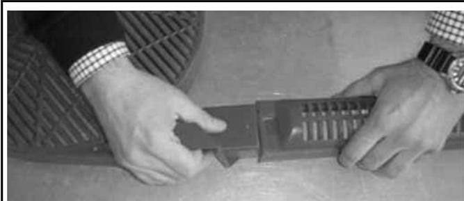
Before assembling the safety meshes complete the Safety-Kit. Join the plastic safety protection for central pulley (ref. 16/a) with plastic safety protection for the v-belt (ref. 16/b).
