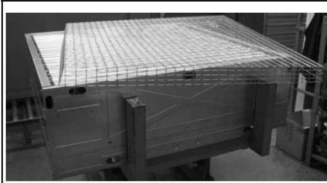
Put the pyramidal shape mesh (ref. 17/a) on the fan as in the picture. The rectangular holes must be positioned horizontally.
