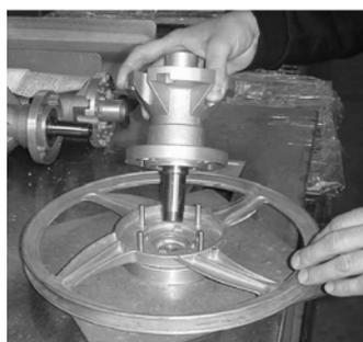
Take the pulley (ref. 10/a) and insert the bolts (ref. 23/a) from the external side of it. Turn the pulley up side down and place the hub (ref. 10/b) on it.
