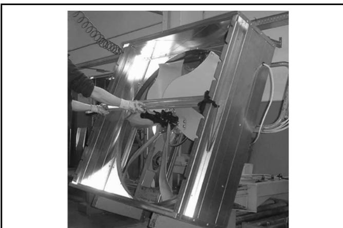
Fit central shutter blade on the central slot on the housing. Insert knurled axle (ref. 30) by the smooth side on the plastic fork, then take plastic shutter rod on the centrifugal system and fix them together by using a small hammer (ref. 38).
