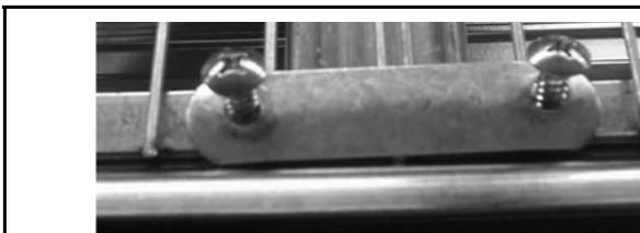
Fix the screws (ref. 32/a) with the central clips (ref.33) in correspondence of the propeller central support on the top panel and the bottom panel.
