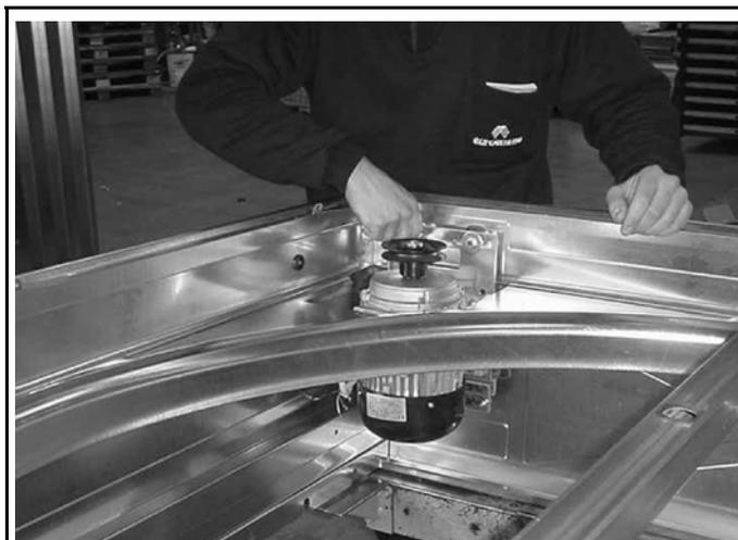
Fix motor slide to top panel by means qty. 2 bolts (ref. 20) and qty. 2 washers (ref. 20). Tighten bolts by using 13 mm spanner (ref. 37).
