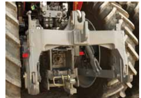
3-point hitch with quick coupler
