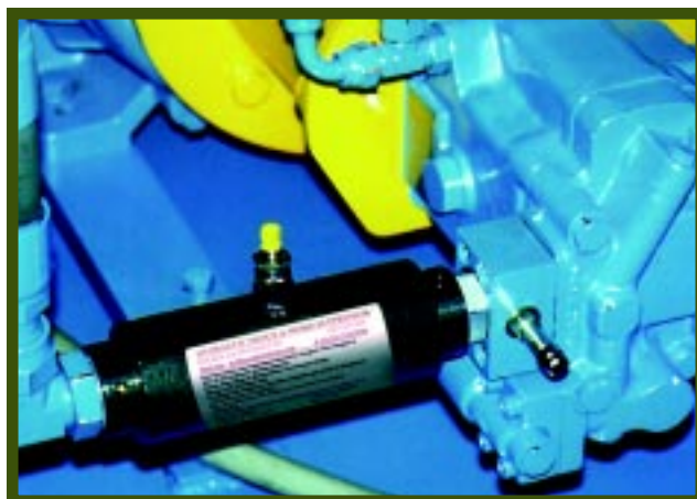
This photo shows a typical installation. The Suppressor shown is only 8.25 inches long so it takes very little space.
