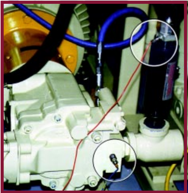
This photo shows the Suppressor mounted at the pump outlet. There are sensors mounted immediately before and after the suppressor leading to the oscilloscope. This is the method used to get the tracings shown below.
