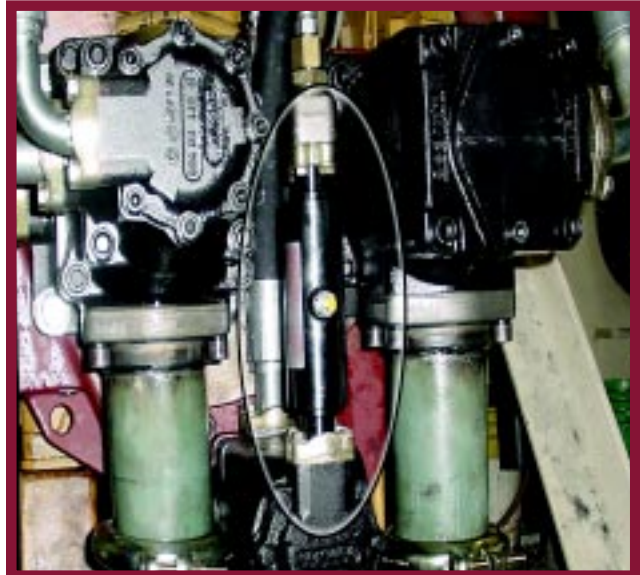
The Suppressor shown is a flange mounted Suppressor at the pump outlet.
