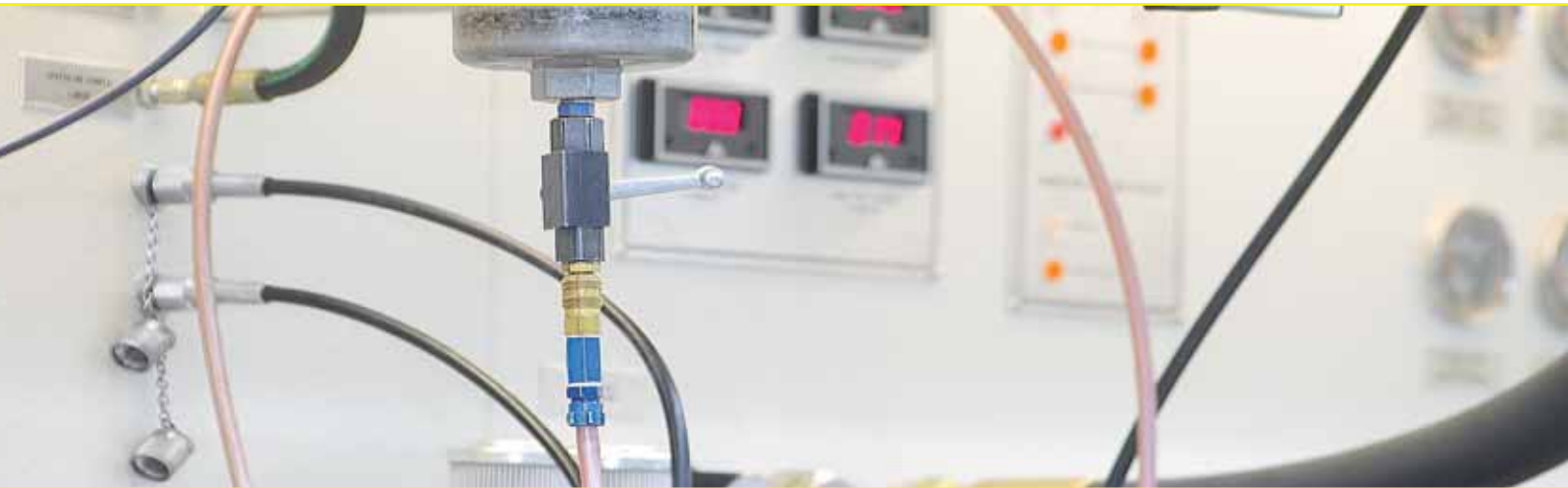
Multipass Test Bench
