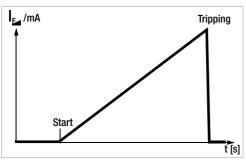
With the selector switch in the I<sub>F</sub> position, slowly rising current flows via N and PE. The momentary measured current value is continuously displayed. When the RCCB is tripped, the last mea-
