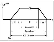
capable of detecting this measuring current, and is consequently not tripped during measurement.
