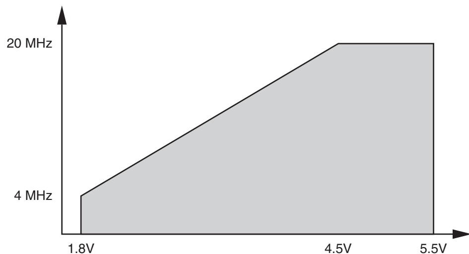
Figure 18-1. Maximum Frequency vs. V_{CC}
