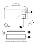
**5** Lubricate the filter element seal with the operating fluid prior to installation (see fig. 4).
