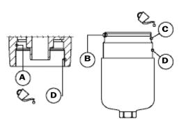
**5** Lubricate the filter element seal with the operating fluid before installing the new filter element (sse fig. 4).
