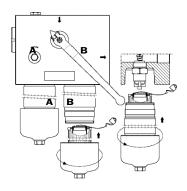
**6** Screw the cover onto the housing (version P01), or the housing onto the head (version P02) using the correct tool. **WARNING:** Screw down the cover / housing fully home into the housing
