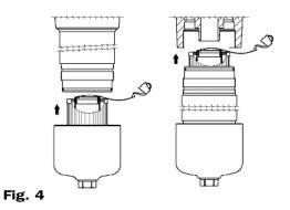
**6** Screw the cover onto the housing (version PO1), or the housing onto the head (version PO2) using the correct tool. **WARNING:** Screw the cover / housing fully home on the housing
