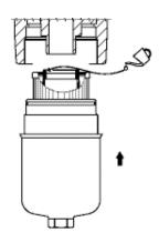
6 Screw the housing onto the head using the correct tool. WARNING: Screw the housing fully home onto the head "DO NOT APPLY EXCESSIVE TIGHTENING TORQUE ".
