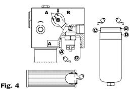
**5** Lubricate the filter element seal with the operating fluid prior to installation.
