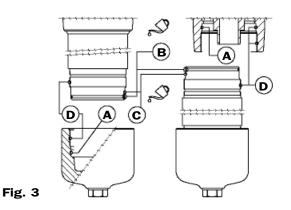
**5** Lubricate the filter element seal with the operating fluid prior to installation (see fig. 4).
