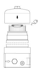
6 Screw the cover onto the housing using the correct tool. WARNING: Screw the cover fully home into the housing "DO NOT APPLY EXCESSIVE TIGHTENING TORQUE ".
