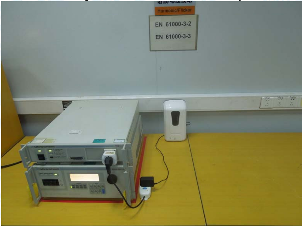
Photo 4 Harmonic current emissions and Voltage fluctuations & flicker Test Setup
