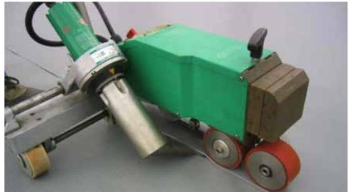
Position the automatic hot air welding machine with the pressure wheel approximately 3 mm over the weld edge to ensure a sealed edge. Lift the overlapping membrane sheet and insert the blower nozzle between the overlap. Immediately begin moving the machine along the lap to prevent scorching of the membrane. The seams are welded in one operation usually at a speed of 2.0 to 3.0 m/min. At the end of the run, remove the nozzle first and then stop the machine's forward motion.
