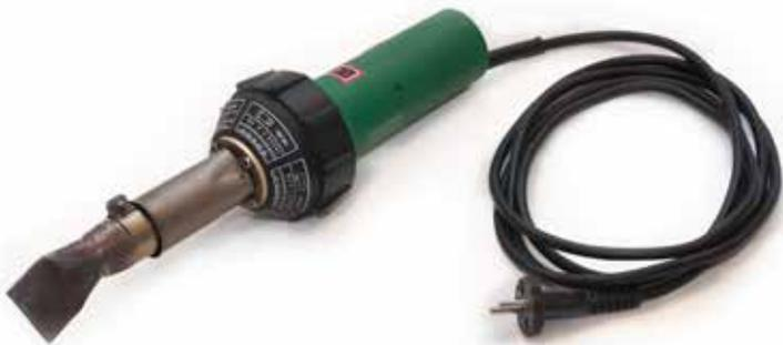
Use a hand-held welder and silicone covered roller to complete welds and details where the welding machine is inappropriate. All hand-held welders, which produce the necessary hot air temperature of approx. 400 - 450 °C and the necessary air volume can be used. Hot-air tools with closed loop controlled temperature (compensation of voltage fluctuations) with display are recommended.
