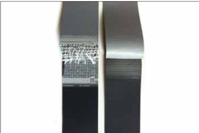
The peel test (by hand) shall not be carried out before the sample has cooled down to ambient temperature. Prior to performing the peel test, cut the sample material into strips 20 mm wide. The samples shall be torn by hand in lengthwise and crosswise direction respectively. When there is a delamination of either the top or bottom sheet the requirement is fulfilled and the welding parameters are set correctly. The delamination means a controlled destruction of the product.
